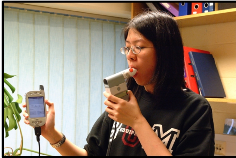
Figure 5.1: A patient with the Vitalograph peak flow meter and O 2 xda used in the Thames Valley Study, the two devices are joined by a customized serial cable.
